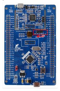
Step 6. When the "Reset" key has been pressed, both LED1 and LED2 will blink as shown on the left side of the following figure. The messages "Hello World! 0" ~ "Hello World! 99" will appear in the "Tera Term" window via the Virtual COM Port, as shown on the right side of the following figure. This is used to verify that it has been successfully used with the Keil MDK-ARM uVision GNU Arm Compiler.
