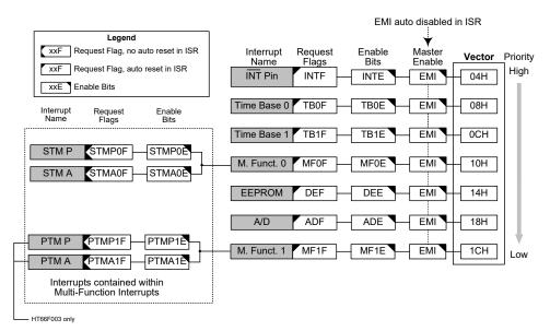
Interrupt Structure - HT66F002/HT66F0025/HT66F003
