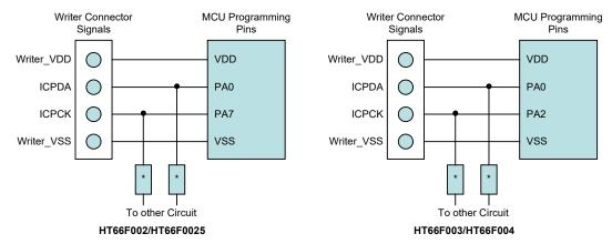
Note: \* may be resistor or capacitor. The resistance of \* must be greater than 1k or the capacitance of \* must be less than 1nF.
