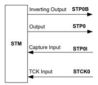
**STM Function Pin Control Block Diagram**
