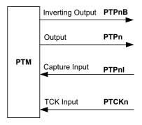
PTM Function Pin Control Block Diagram
