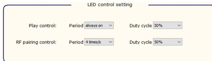
The screenshot shows a settings window titled "LED control setting". It contains two rows of controls. The first row is for "Play control:" with a "Period" dropdown set to "always on" and a "Duty cycle" dropdown set to "50%". The second row is for "RF pairing control:" with a "Period" dropdown set to "4 times/s" and a "Duty cycle" dropdown set to "50%".
