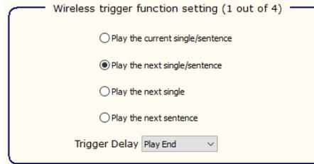
Set the voice playback mode when receiving RF trigger.
