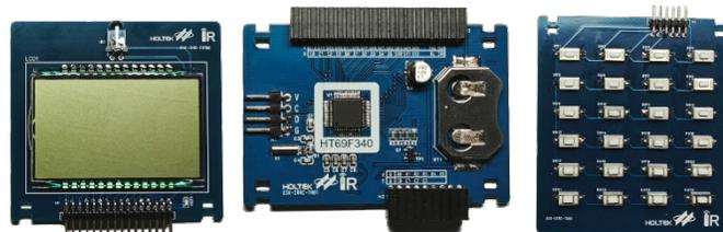
**Modular LCD Remote Controller Development Board**
