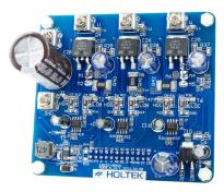
Medium Voltage Power Board (MVPB) Input voltage: DC 17V to 60V Maximum DC bus current: 20A
