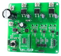
Medium Voltage Power Board (MVPD with integrated MCU) Input voltage: DC 15V to 60V Maximum DC bus current: 20A
