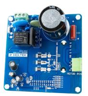
High Voltage Power Board (HVPB) Input voltage: AC 90V to 264V Maximum DC bus current: 2.5A
