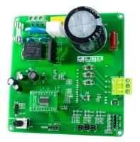
High Voltage Power Board (HVPD with integrated MCU)
